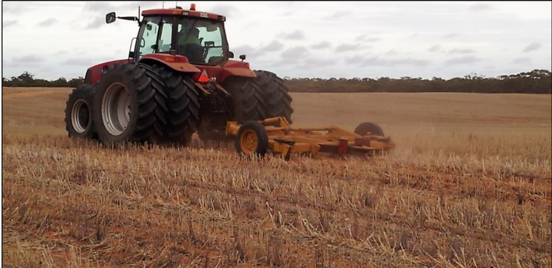
Figure 6. Deep ripper in action showing maintenance of surface stubble cover
