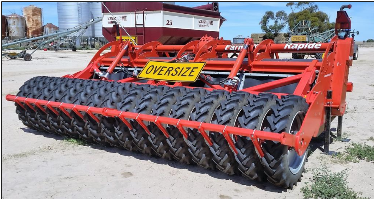
Figure 29. Spading machine with large presswheels to leave ground ridged and firm
