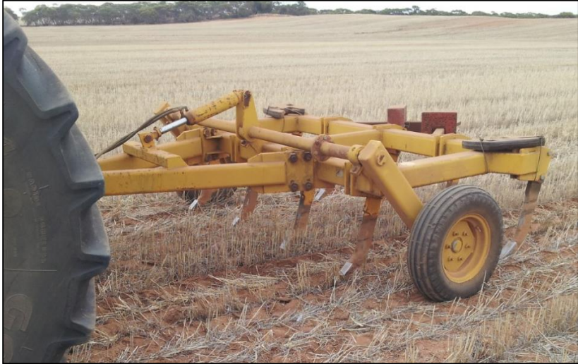
Figure 6. Deep ripper in action showing maintenance of surface stubble cover
